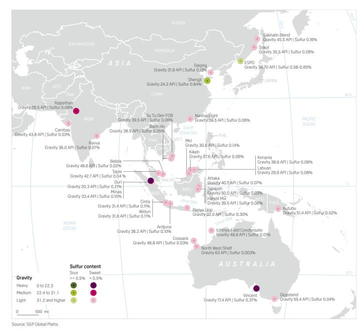
Attaka: The assessments reflect Attaka crude cargoes for lifting on a FOB basis from the Santan oil terminal, Indonesia. Attaka crude is produced offshore East Kalimantan. It has a typical API gravity of 40.66 with a sulfur content of 0.07%.
